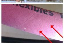
The hose is beyond its serviceable life and showing signs of degradation. Considering the criticality of this hose to production, the hose should be replaced at the next available maintenance interval.
